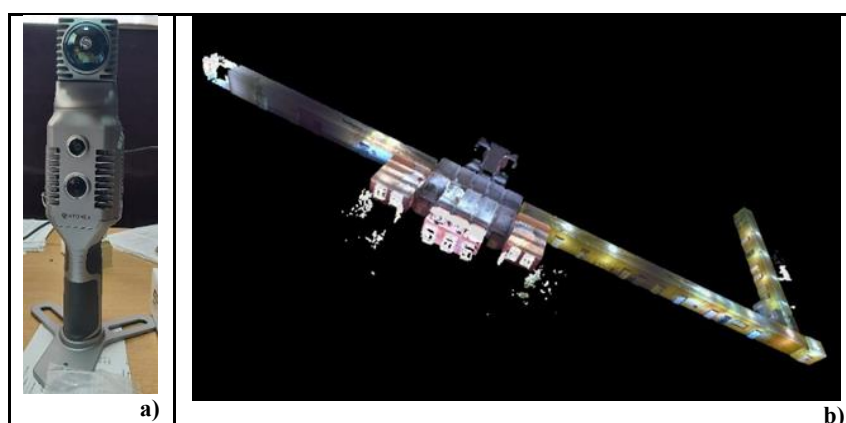
Figure 1. A fragment of the scanning results when using a handheld 3D scanner a) handheld 3D scanner b) 3D model
