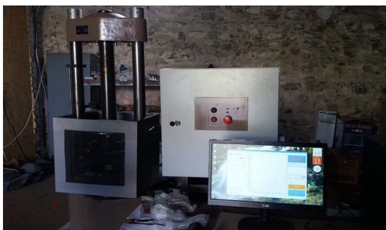
Figure 2. The strength of uranium ore samples was tested using a hydraulic press
