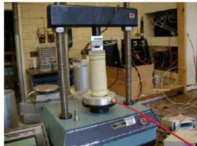
Figure 5 - Sample set on loading frame.
