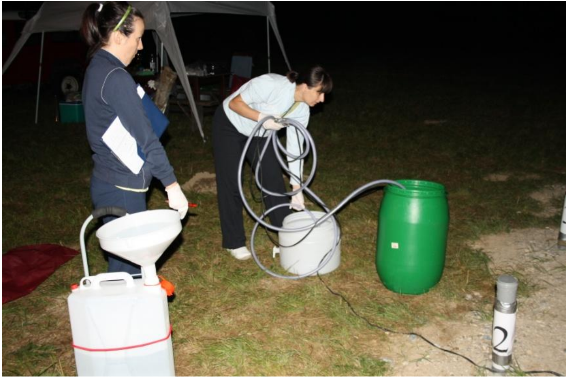
Figure 12 Cleaning of the pump after each sampling
