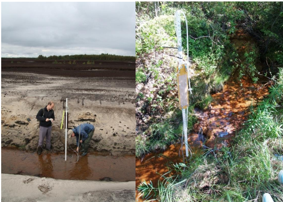
Fig. 3.11 Use of potentiomanometer in a small streams located at peat production area (left) and groundwater discharge area (right) to determine the direction of water seepage.
