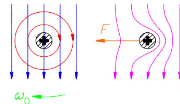
zbog  $I_{20}$  i  $\Phi \Rightarrow F \Rightarrow M \Rightarrow$  vrtnja rotora  $\Rightarrow \downarrow f$  induciranog  $U$  u rotoru
