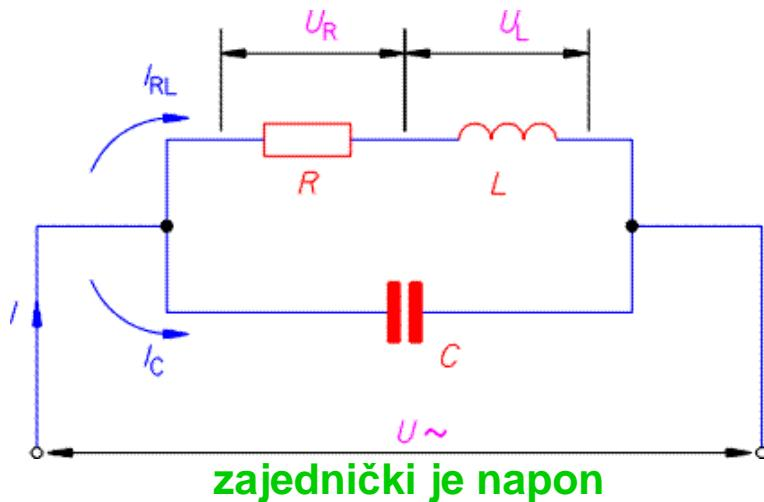
$$I_{RL} = \frac{U}{R + j\omega L} \quad U = I_{RL} \cdot R + jI_{RL} \cdot \omega L = -U_{\sim}$$
