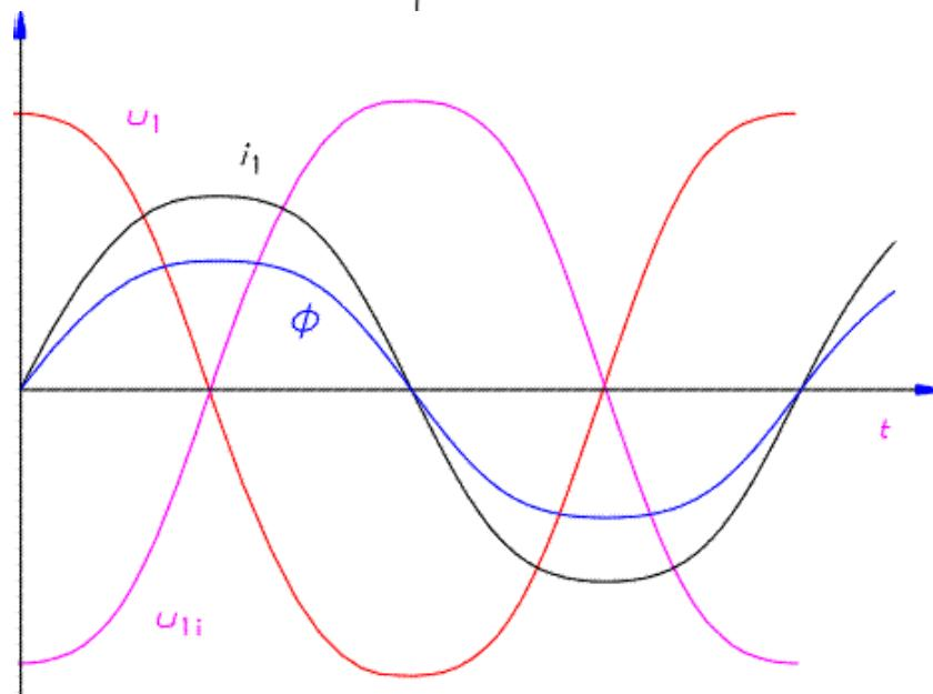
$$\begin{aligned} u_i &= -\frac{d\Phi}{dt} = -\Phi_{max} \cdot \frac{d(\sin \omega t)}{dt} \\ &= \omega \cdot \Phi_{max} \cdot \sin\left(\omega t - \frac{\pi}{2}\right) \end{aligned}$$
