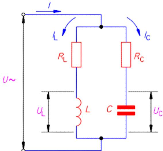
$$\omega_0 = \left( \frac{R_L^2 - \frac{L}{C}}{LCR_C^2 - L^2} \right)^{\frac{1}{2}} = \frac{1}{\sqrt{LC}} \left( \frac{R_L^2 - \frac{L}{C}}{R_C^2 - \frac{L}{C}} \right)^{\frac{1}{2}}$$
