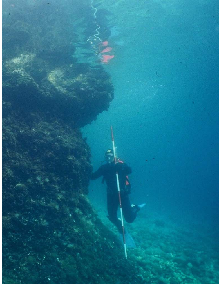
Fig. 6. Tidal notch formed in Cretaceous rudist limestones on the northeastern coast of Rijeka Bay, the roof is 0.37 m below BMSL, local tidal range is approximately 0.5 m (location 13, N=501715 ; E=546064 ; Photo: D. Frka, Sept. 1998).
